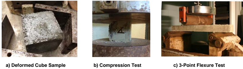
Figure 6. Compression and flexure tests of sulphur concrete mixes
